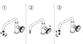
5. Remove the aerator with the key and turn on faucet for 1 minute to flush debris from faucet and feed lines. Turn off faucet and re-install the aerator with the key.
