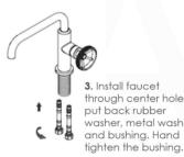
3. Install faucet through center hole, put back rubber washer, metal washer and bushing, Hand
